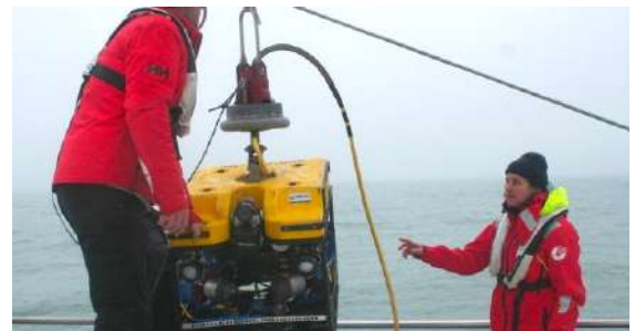
ROVs have been deployed from the Sea Ranger Service ship for surveying offshore installations in the North Sea.
